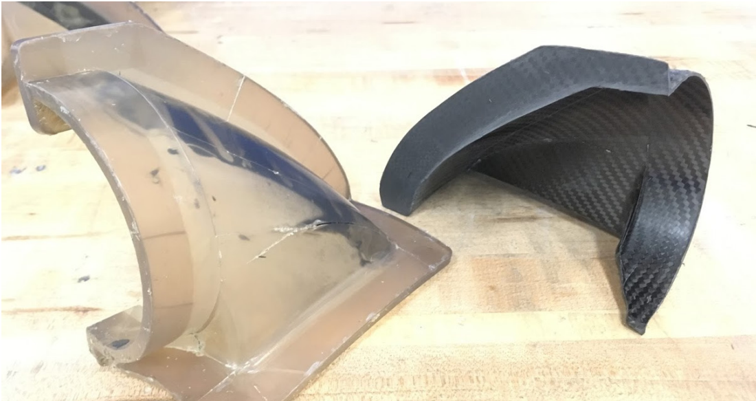
The left half of the carbon fiber duct (right) demolded from the 3D printed mold covered in Kapton tape (left).
