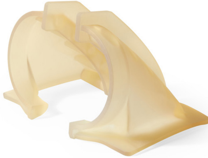
The two-parts mold printed with High Temp Resin.
