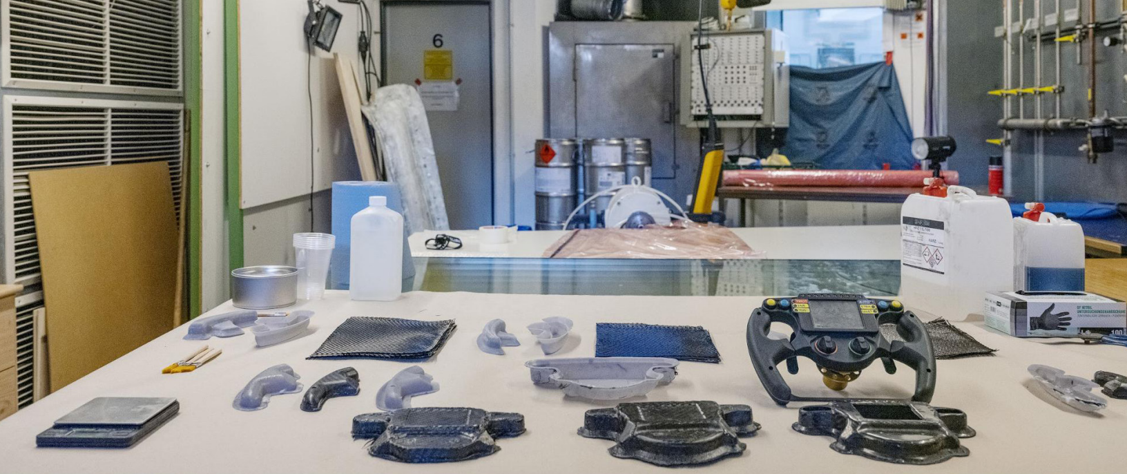
The FaSTTUBe test bench with the carbon fiber parts manufacturing set up.
