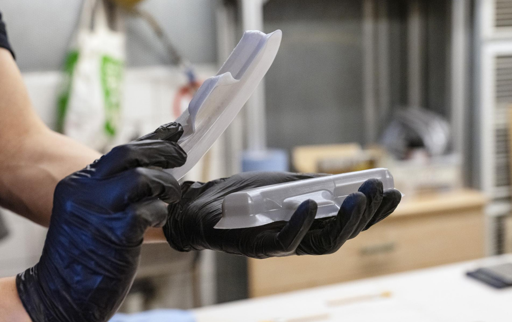
The two-parts mold of the grip steering wheel printed with Tough 1500 Resin.
