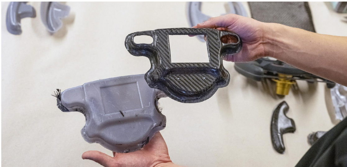
The 3D printed mold and the demolded carbon fiber part for the steering wheel front housing.
